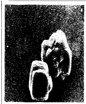
Figure 11C—Polyacrylate (2000x, 12-18 microns)
