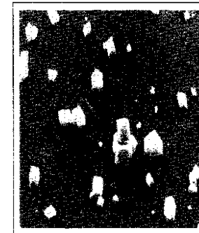
Figure 11A—Untreated \text{CaCO}_3 (calcite 2000x, 4 microns)
